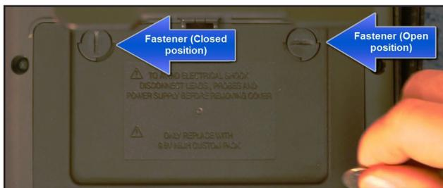
Using a flat screwdriver or equivalent, gently remove the cover from the compartment, taking care not to damage the plastic cover holder.
