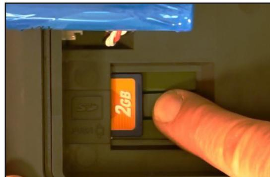
Remove the SD card, and locate the write-prevention slider on the left edge of the card. When the card is first removed from the instrument, it is in the unlocked position (the slider is positioned towards the card’s metal pins). To prevent the card from accidentally being overwritten during the download procedure, you must move the slider to the LOCK position (see below). The LOCK direction is away from the metal tabs on the SD card.
