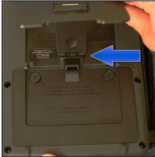
Locate the two fasteners on the battery compartment cover. Using a coin or similar implement, turn each fastener 90° counterclockwise (the fastener slot will now be in the horizontal position).
