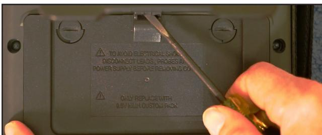
Turn the instrument over and hold the battery as it slides out of its compartment. Position the battery out of the way, but do not unplug it.
